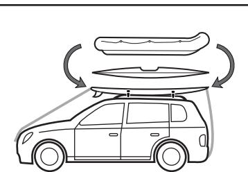
(EN) Any load extending over the windshield (except roof baskets) must be secured to both the front and rear of the vehicle, in addition to the rack. Failure to do so may result in property damage, personal injury or death.
