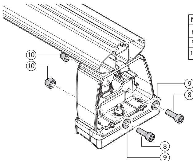
EN) To facilitate assembly, keep the nut pressed in the dedicated seat.
