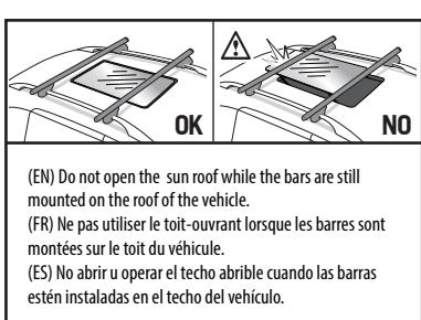
(EN) Do not open the sun roof while the bars are still mounted on the roof of the vehicle.
