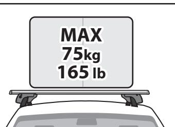
(EN) Do not exceed the maximum load specified for the roof rack, accessory rack or the maximum load recommended by the vehicle manufacturer. **Max roof load = weight of the complete roof rack system + weight of the load**
