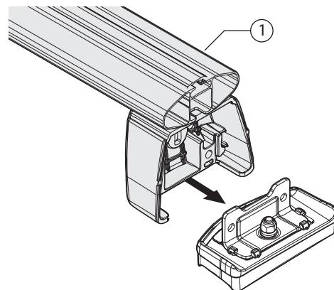
EN) Tighten the screws manually before proceeding with the final tightening.
