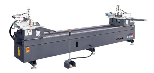
**APEX - II,** which has automatic hydraulic double head corner crimping, is used for corner binding processes for aluminium profiles. Incorporating manual metering precision and the power of hydraulic system in its body, it provides its users with quick solutions.
