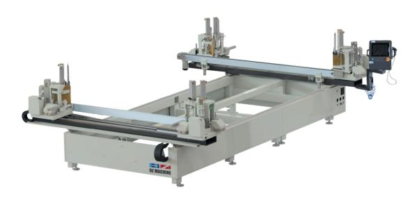
**ORION - IV** which is quadruple welding center has been developed for welding 4 edges of plastic profiles process. Through its electronic thermostat provides to be boiled at the same time of 4 edges by scattering homogenised to plaque of heat with adjustable welding time and intended heat value between 0 °C - 350 °C. **ORION - IV** which has process programming and wide memory capacity enables data transfer on distant network connection, Ethernet and USB.
