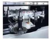
High speed rates on axes and internal automatic tool replacement magazine which moves with gantry for 10 tools allow for time savings when running different processes which require tool replacement.
