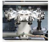
High speed rates on axes and internal automatic tool replacement magazine which moves with gantry for 10+1 tools allow for time savings when running different processes which require tool replacement.
