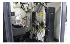
7 units of fan cooled spindle motors that can function and be positioned as different angles enables an unlimited operational capability on 4 surfaces of the profile.
