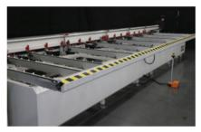
Thanks to the feeding capacity of 10 profiles, the conveyor structure enables batch processing, letting the machine to be used in the most efficient manner.
