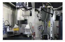
The cutting unit with a 550 mm diameter saw blade for cutting at every angle between 30° and 150° offers a wide cutting range to users.
