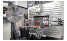
8 fan-cooled spindle motors which can operate at different angles, offer unlimited processing on 4 surfaces of the profile.
