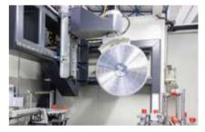
550 mm diameter saw that can cut at any angle between 0° and 180° thanks to its 4-axis movement capability, the saw allows cutting and end-milling operations of profiles up to 300 mm wide.
