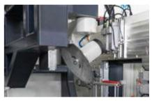
550 mm diameter saw that can cut at any angle between 0° and 180° thanks to its 5-axis movement capability, the saw allows cutting and end-milling operations of profiles up to 300 mm wide.
