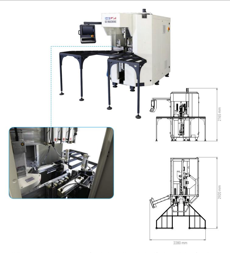
**ORBIT - V,** the Automatic PVC corner and surface cleaning machine, is developed for cleaning the burrs formed on the plastic profiles after the process of welding. Cleans the lower, upper, inner and outer surfaces of profiles by means of two independent cleaning units. 11 automatic profile cleaning blades provide the users with ease and time saving in burr cleaning process with its 1000 pcs. profile memory capacity and operator adjustable axial speeds.
