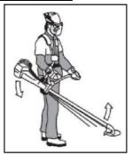
Lower cutter to ground contact & adjust suspension point for balance
