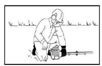
Place the unit on the ground: It must rest securely on the engine support and the detector. Check that the cutting attachment is not touching the ground or any other obstacles.
