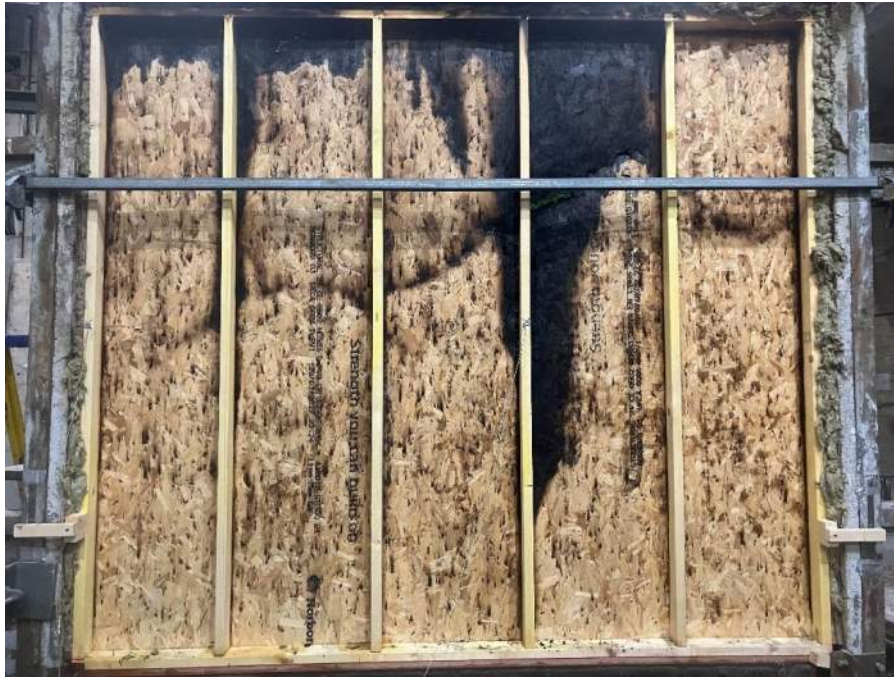
Figure 25 Unexposed face of the specimen after the test
