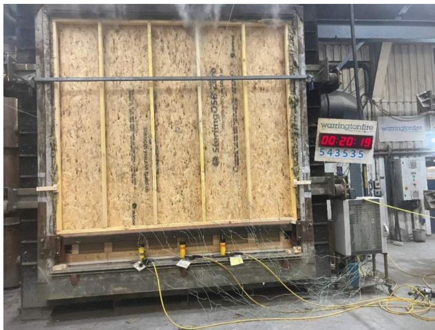
Figure 21 Unexposed face of the specimen after 15:00 minutes of testing
