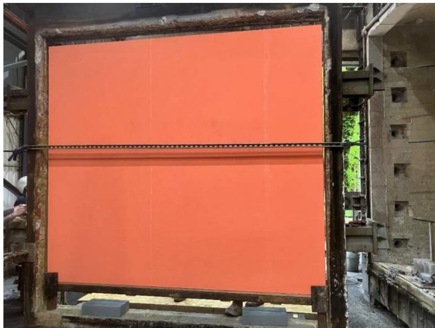
Figure 18 Exposed face of the specimen before the start of the test (support bar and clamp removed prior to fitting onto furnace)
