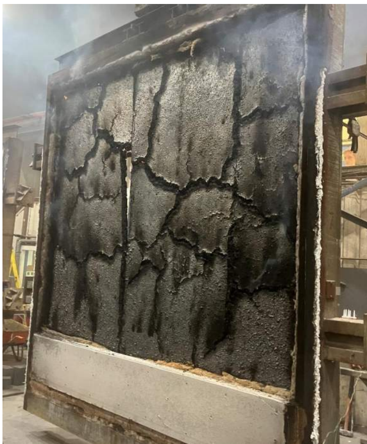
Figure 25 Unexposed face of the specimen after the test
