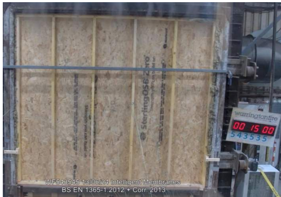
Figure 21 Unexposed face of the specimen after 15:00 minutes of testing
