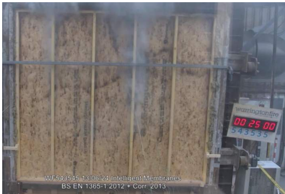
Figure 23 Unexposed face of the specimen after 23:19 minutes of testing
