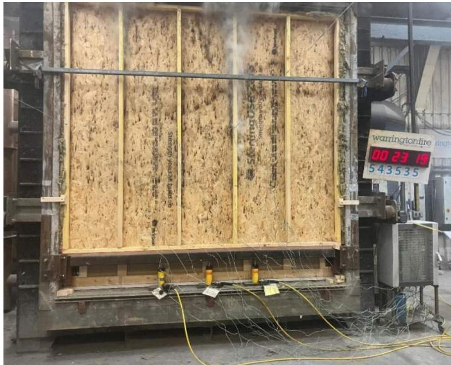
Figure 23 Unexposed face of the specimen after 23:19 minutes of testing
