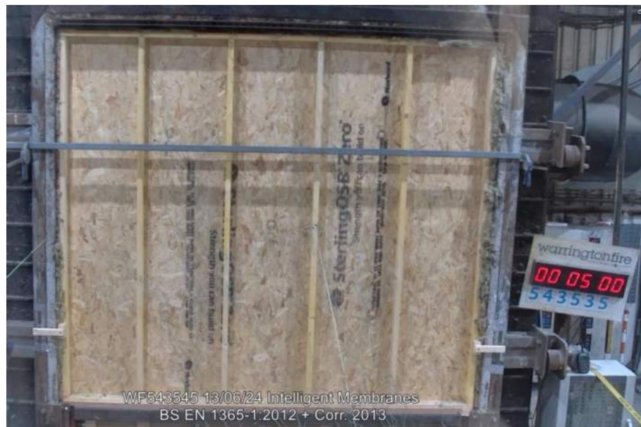
Figure 19 Unexposed face of the specimen after 05:00 minutes of testing
