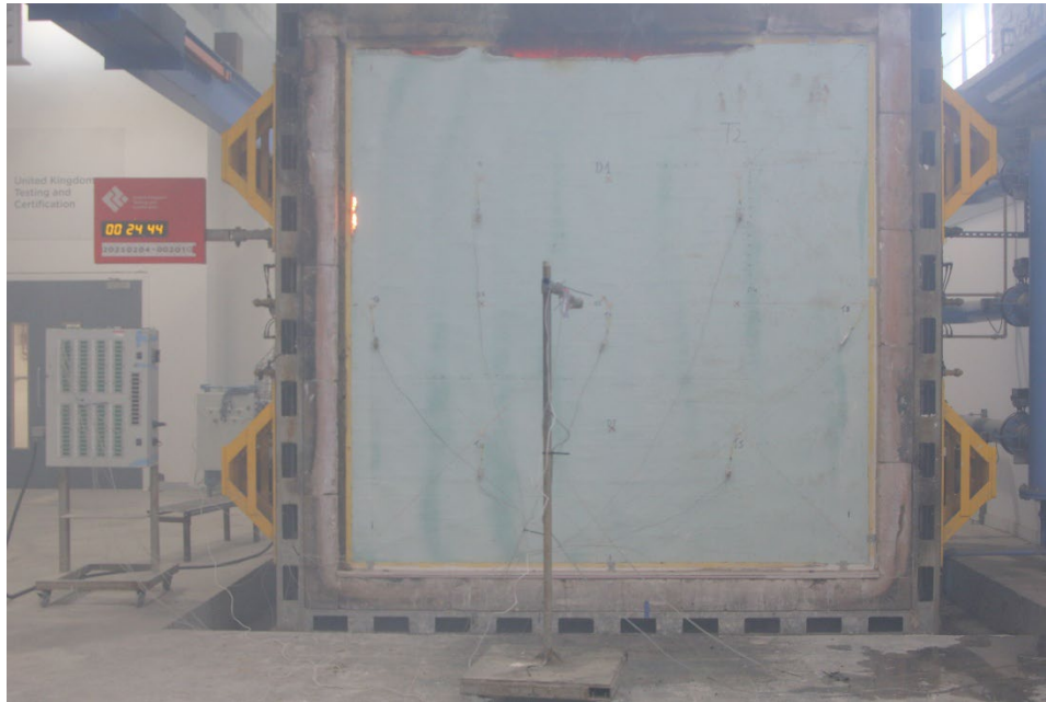
Figure 18 - The unexposed surface of the test construction after a test duration of 24 minutes
