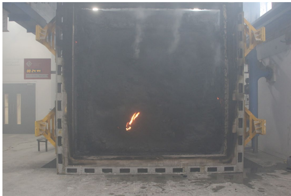
Figure 19 - The exposed surface of the test construction after the test was discontinued
