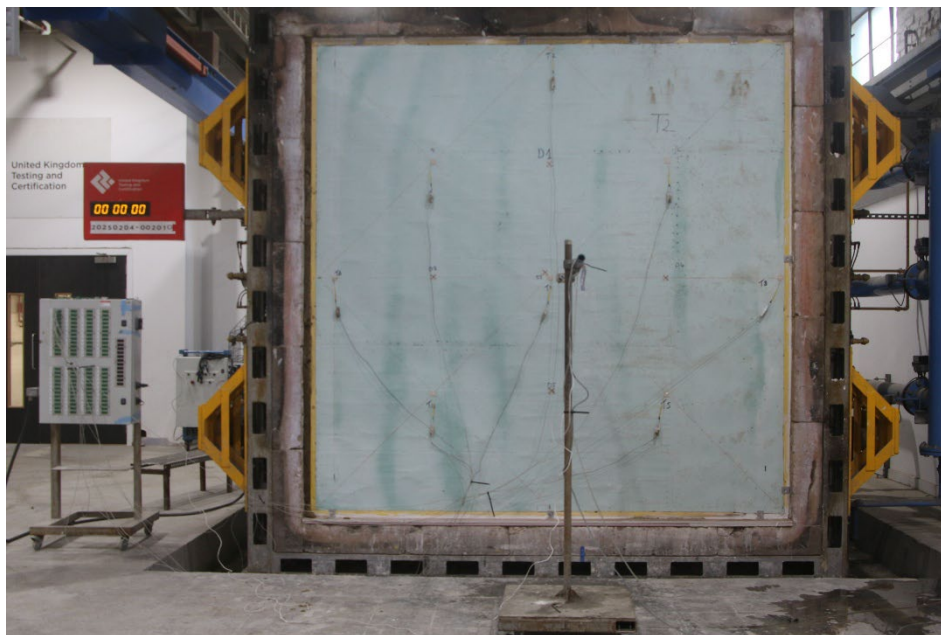
Figure 15 - The unexposed surface of the test construction prior to the commencement of the test
