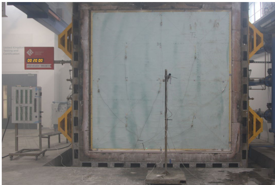
Figure 17 - The unexposed surface of the test construction after a test duration of 20 minutes
