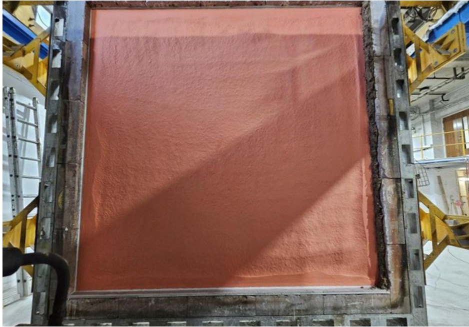
Figure 14 – The exposed surface of the test construction prior to commencement of the test
