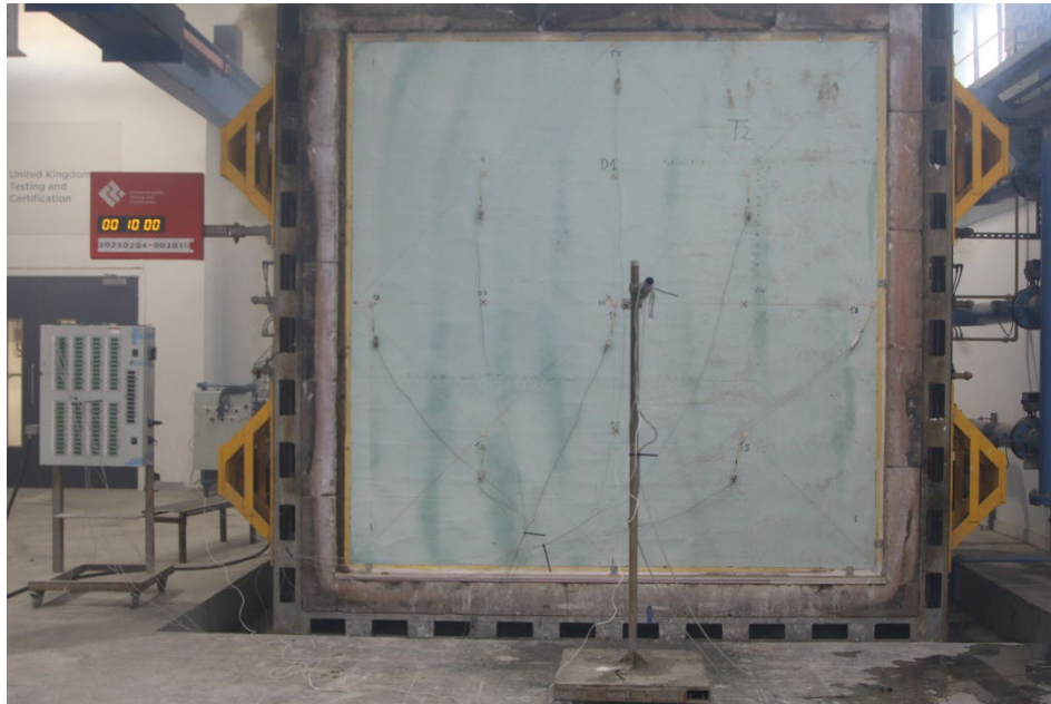
Figure 16 - The unexposed surface of the test construction after a test duration of 10 minutes
