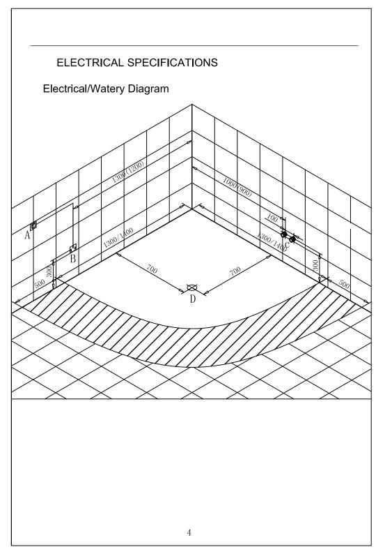
The power cable should be installed with leakage protector and connected to the ground. The cross section area of power cable should at least 2.5 square mm or above. The power supply facility should conform to national safety standard (please prepare the leakage protective switch by yourself), and the protective ground wire should be connected with the massage bathtub iron hob, where there is a symbol for ground wire.
