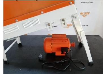
6. Attach the drive belt to the position, after which the engine pulley is aligned with the pulley of the drum. Fix the engine, by firmly tightening the screws.
