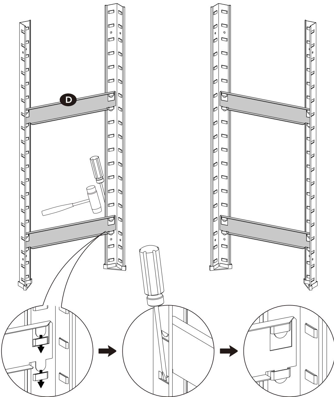
**EN** Insert both of the part D clips into the two slots of part B and make sure both of the clips pass entirely through the slot with its tip coming back out to the front to form a firm joint.
