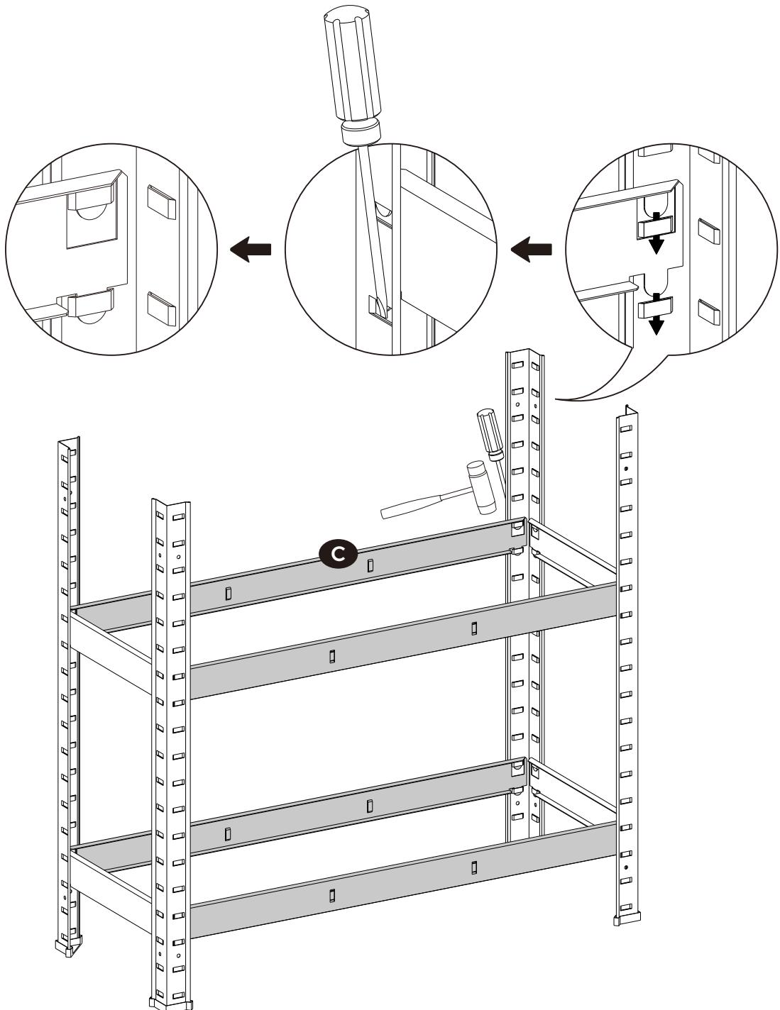
**EN** Insert both of the part C clips into the two slots of part B and make sure both of the clips pass entirely through the slot with its tip coming back out to the front to form a firm joint.
