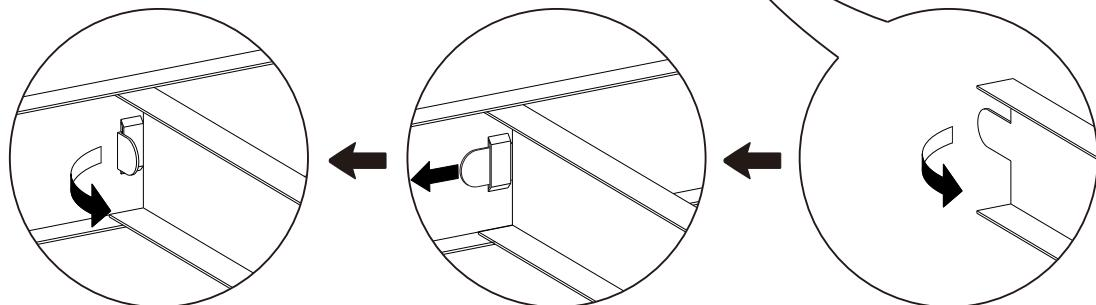
**EN** Bend the clip of part F to 90 degrees and insert the clip to the slot at the middle of part C, then bend the tip part of the clips to 90 degrees for a tight joint. This is to ensure that part F doesn't come off from part C.
