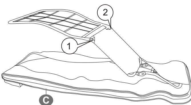
Note: Label 1 should be on the outside when putting the cover over the metal frame.
