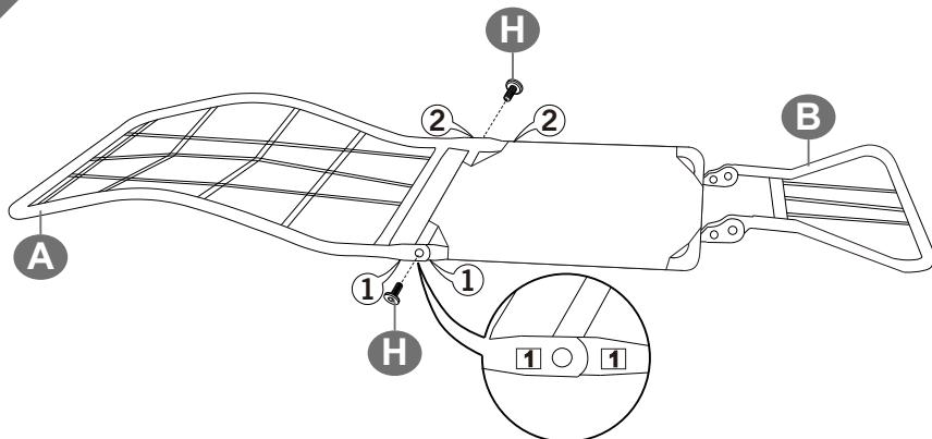
Note: Label 1 on Part A and Part B should be on the same side as shown.
