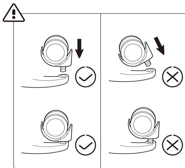
make sure that the axle of the wheel is fully inserted.
