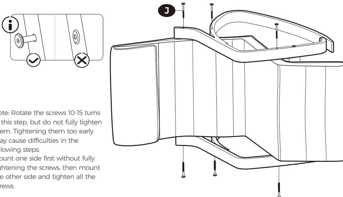
**EN** Note: Rotate the screws 10-15 turns in this step, but do not fully tighten them. Tightening them too early may cause difficulties in the following steps.
