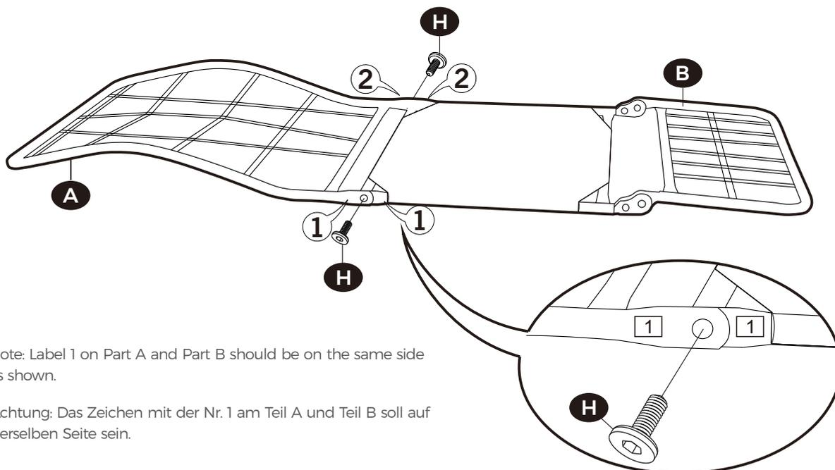
**EN** Note: Label 1 on Part A and Part B should be on the same side as shown.
