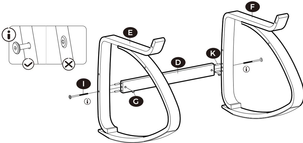
**EN** Note: Rotate the screws 7-8 turns in this step, but do not fully tighten them. Tightening them too early may cause difficulties in the following steps.
