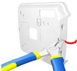
Figure 2: Surface-mount cabling plastic tab removal
