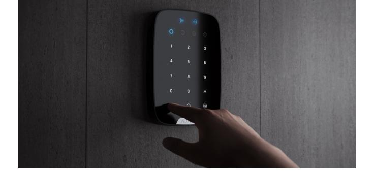
You can activate the keypad by swiping your hand over the touch panel from top to bottom. When activated, the backlight on the keypad will turn on and a beep will sound (if enabled).
