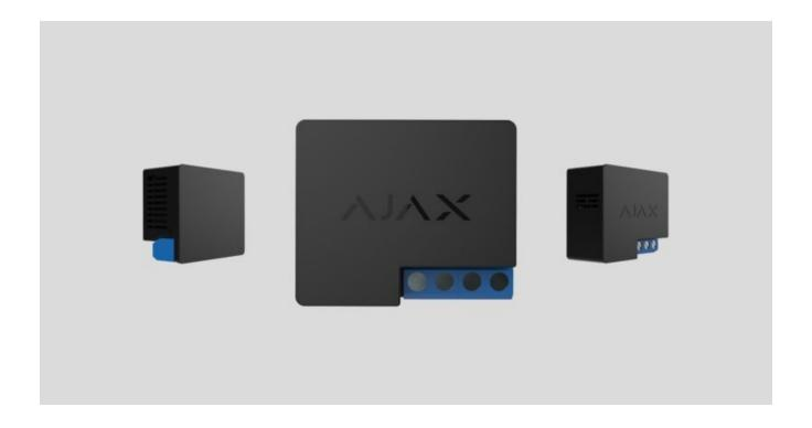
**Relay** is a wireless, low-voltage relay featuring potential-free (dry) contacts. Use Relay to remotely switch on/off appliances powered by a 7–24 V DC source. Relay can operate both in pulse and bistable mode. The device communicates with a hub via <u>Jeweller</u> radio protocol. In the line of sight, the communication distance is up to 1,000 m.
