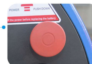
Emergency Power-off Switch
