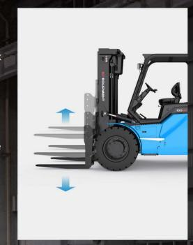
The high-capacity forklift mast is equipped with a hydraulic buffering system that ensures smooth lifting and lowering of loads. With controlled deceleration, the fork movement is smooth with no abrupt stops that could damage the load or cause operator discomfort. This feature enhances operational safety and prolongs the lifespan of the mast components.
