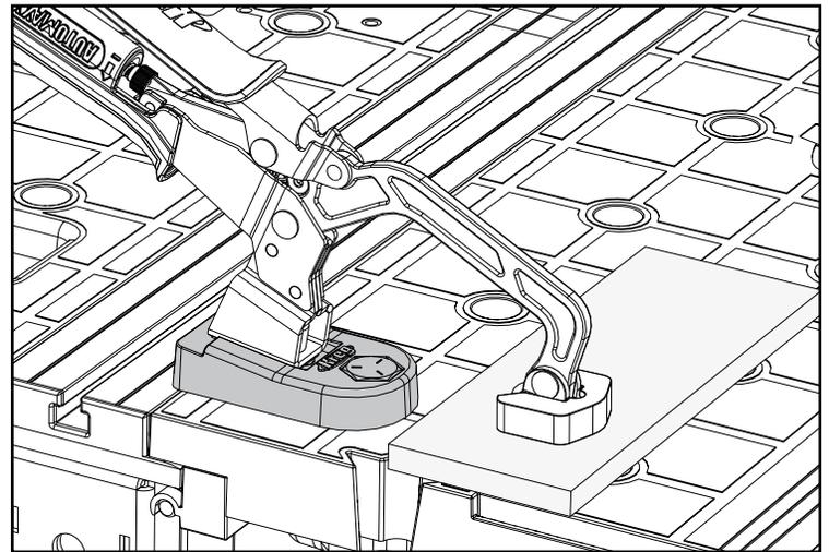
With the Bench Clamp Base mounted on your Kreg Mobile Project Center table top or workbench, tighten the knob so it is snug, not tight. This allows the Clamp Base to pivot for optimum alignment with the workpiece. Adjust the Bench Clamp bolt as shown and test the fit of the Bench Clamp in the Clamp Base keyhole slot. The Bench Clamp should be snug but slide easily. Never allow the Bench Clamp Bolt to become loose enough to allow the Bench Clamp to pivot outside of the Clamp Base recess.
