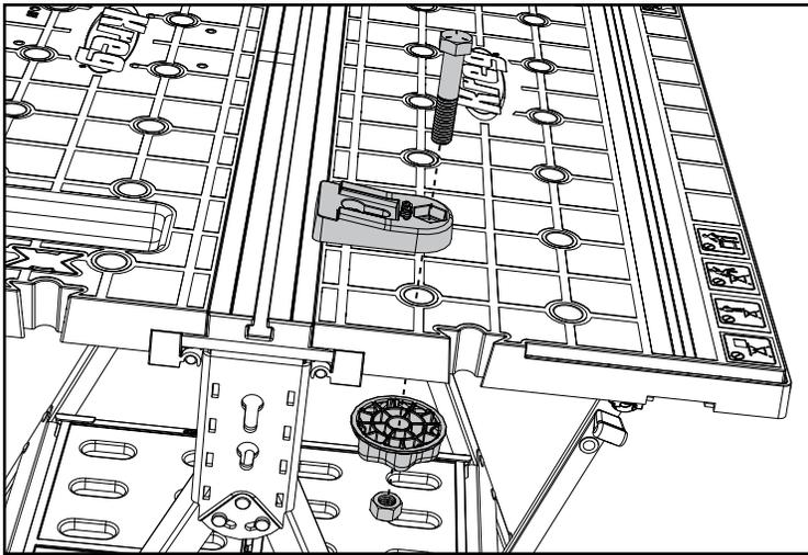
Assemble the Bench Clamp Base as shown. Align the hex nut with the recess in the knob and tighten the knob, seating the nut in the recess. The nut stays in place for future use.
