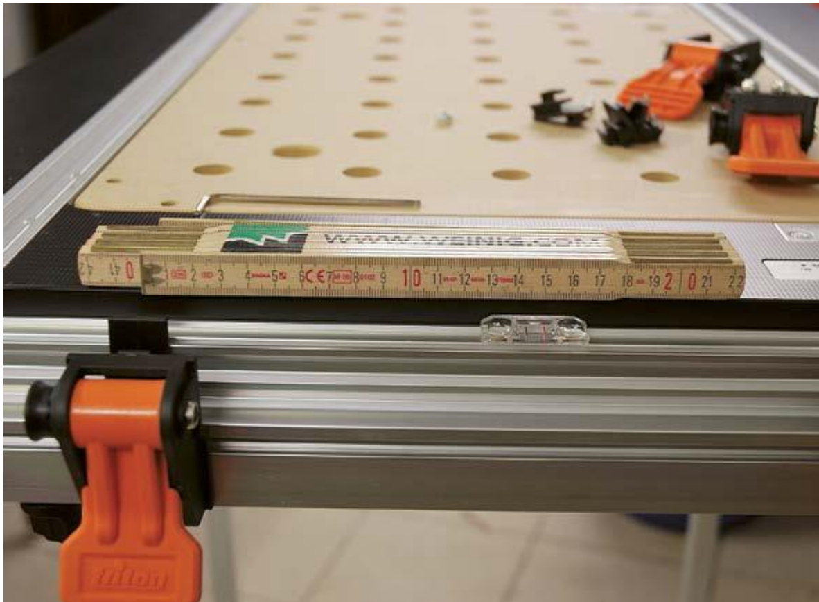
Aluminium extruded side rails perfectly align with the saw blade.
