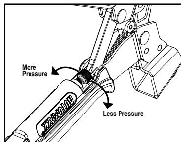
To increase clamp pressure, turn the knurled-head screw to the left (viewed from the handle-end of the clamp); for less pressure, turn the screw to the right.
