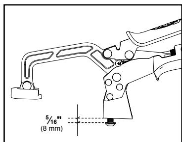
Adjust the anchor screw to leave  $\frac{5}{16}$ " [8mm] between the screw head and the glide pad adhered to the clamp base. Test the fit of the Bench Clamp in the Clamp Plate keyhole. Adjust the screw as necessary until the clamp is snug to the plate but still moves freely in and out of the keyhole. The patch of thread-locking compound on the screw keeps it in position.
