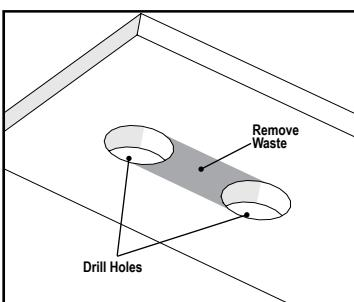
To provide clearance below the Clamp Plate for the anchor screw head, place the plate in the recess and trace the outline of the keyhole onto the bottom of the recess with a pencil. Drill a  $\frac{3}{4}$ " [19mm] hole  $\frac{1}{4}$ " [6mm] deep at each end of the traced outline. Remove the material between the holes with a chisel. Place the plate in the recess and make sure the Bench Clamp anchor screw moves freely in the keyhole.
