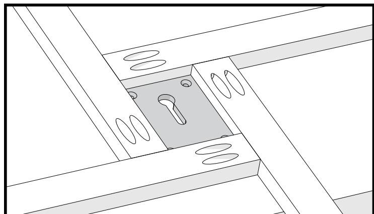
Cut four routing guides from pieces of  $\frac{3}{4}$ " [19mm] stock wide enough to accommodate two pocket screws and long enough to clamp to the surface being routed without interfering with the router. For a smooth-bottom recess, make sure the four guides are the same thickness. Drill pocket holes in one end of each guide. Position the guides around the Clamp Plate as shown, making a snug fit. Drive the pocket screws.
