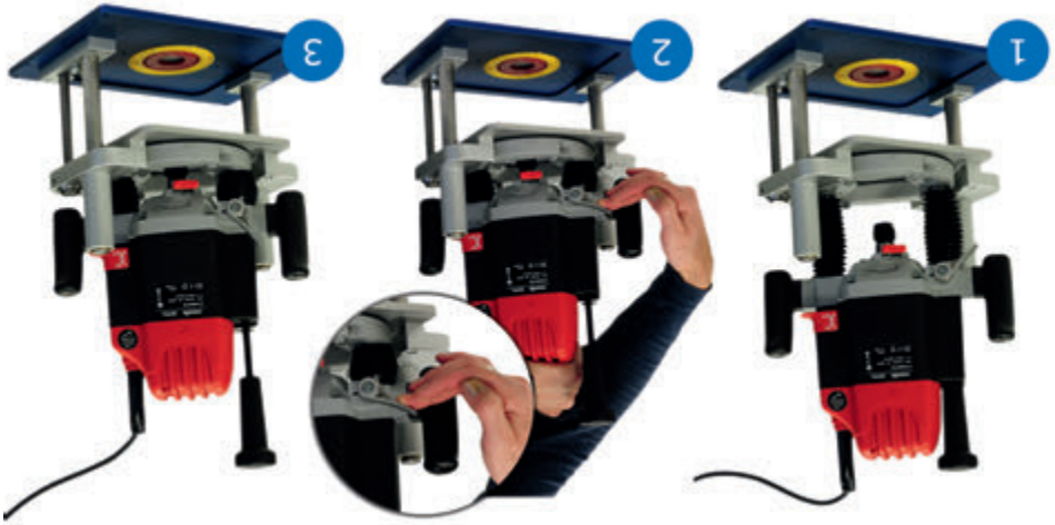
Fig. 8 Minimizing the milling height loss
