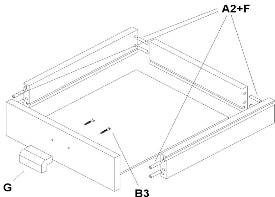
**!!! HINT 1 !!!** - don't fill up holes for dowels by glue. Smear dowels by glue and insert them into holes.
