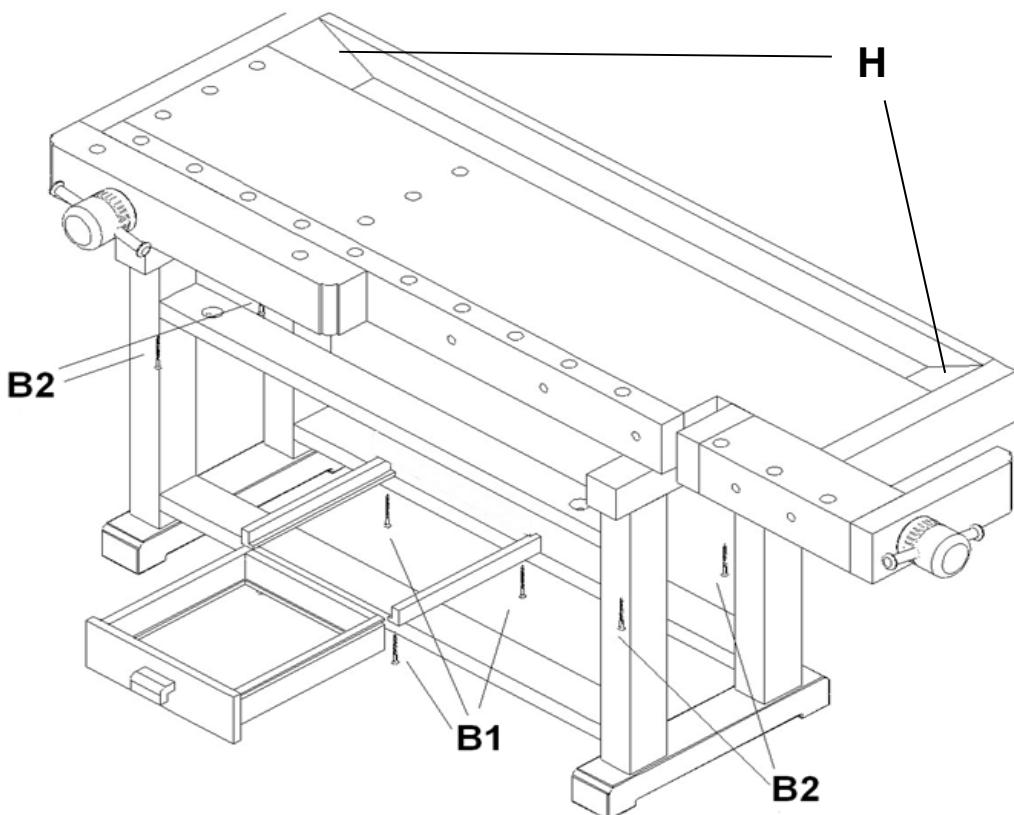
**Important!** Wedges for tool well are supplied separately (part H). Producer recommends to add wedges after approx. 4 weeks. Workbench needs to adapt to the surrounding conditions. In case of need adjust the size of wedges by size of tool well.
