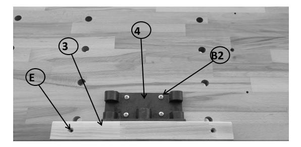
Sand the edges of the wooden jaw face (3) with sandpaper. Fix the wooden jaw face (3) with 5x80 mm screws (E) in the pre-drilled holes. Unscrew the spindle (4) from the spindle body and use 6x30 mm screws (B2) to fix it to the wooden jaw face according to the pre-drilled holes.
