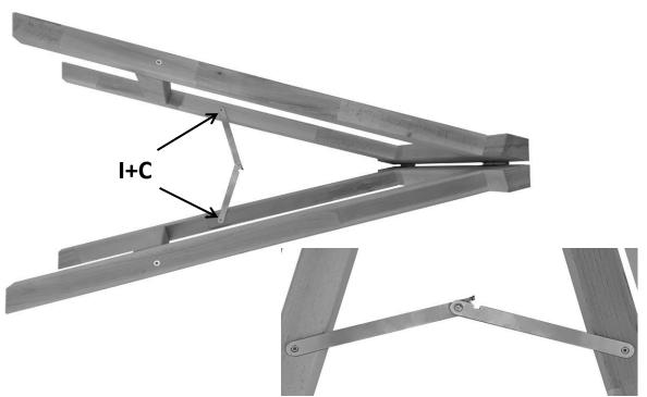
Fix the braces (I) to the legs with the 3x16 mm screws (C). The stops on the Ramia s.r.o., Zátaví 58, CZr397.01+ Písek, Czech Republic, Tek: +420.382r264c450c fax: i+420.382r264 450, www.ramia.cz
