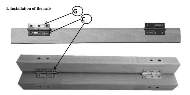
Join the rails (7) using hinges (G) and screws (C). WARNING!!! The package contains 2 types of rails. 2 pieces with dowel holes (locking plate) and 2 pieces without holes. Each saw horse must have one rail with a dowel hole. The cutouts in the rails must point downwards. The dowel holes in the saw horses must face each other.
