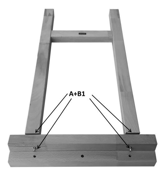
Install the joined right and left leg on the assembled rails using dowels (A) and flat-head furniture screws (B1). The right legs and rung with logo must be on the rail without the hole for the dowel, and the left leg with rung without logo must be on the rail with the hole for the dowel.
