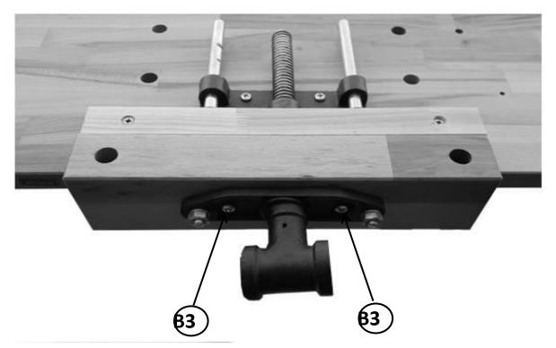
Fully tighten the wooden jaw (2) with the spindle and ensure that it is horizontal with the table top. After this, fix the wooden jaw with 6x40 mm screws (B3) to the spindle guide.
