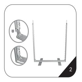
Assemble the frame by connecting the parts with matching numbers & connect wires
