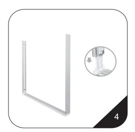
Assemble the top half of the frame by connect the parts with matching numbers
