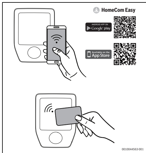
Fig. 48 Authentication via RFID card
