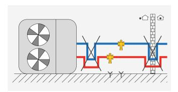
Freezing protection valves must be installed:
