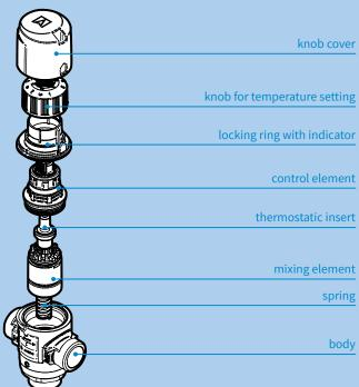
The drawing with the construction of the ATM valve is shown only for illustrative purposes. Please do not disassemble ① the valve. This may lead to improper work and scalds.
