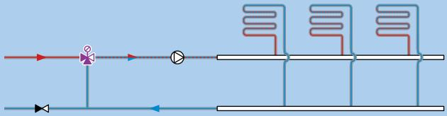
The **ATM** mixing valve presented on the scheme prepares the supply medium for the underfloor heating system. One can use an **ATM** valve with different Kvs values. For manifolds with more than 5 circuits we recommend valves with minimum 2,5 m³/h Kvs. Adding the non-return valve as shown on the scheme will prevent from taking water from the return side and stop gravity flows when the pump does not work.
