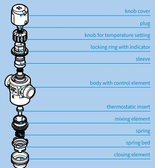
The drawing with the construction of the **ATM** valve is shown only for illustrative purposes. Please do not disassemble the valve. This may lead to improper work and scalds.
