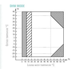
Operating range of heat pump with possible limitation and protection
