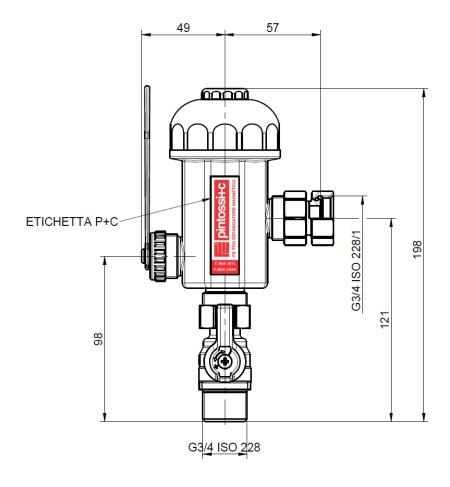
Installation It is recommended to install the filter on the return circuit, before the fluid enter the boiler.
