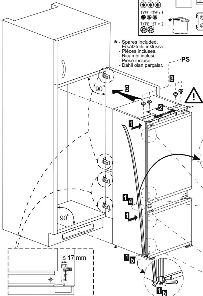
**Note:** Installation step for 2, screws for connecting top plastic part should not be screwed very hard, because of moving the plastic part easily left or right side.
