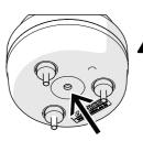
When installing display light with built-in buzzer, make sure to maintain the space (gap) between the installed side and base body at least maximum 5mm or above.
