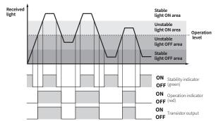
· In Dark ON mode, the waveforms are reversed.
