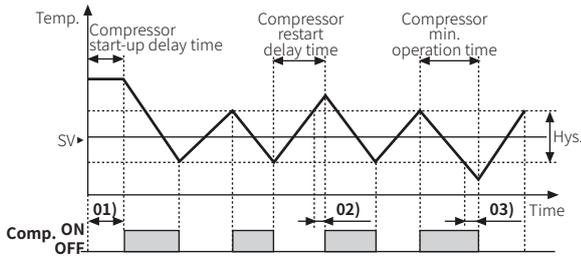
01) When starting compressor, if PV is out of hysteresis range, compressor output does not turn ON and the COMP indicator is flashing during compressor start-up delay time.
