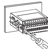
Mount the product to panel with bracket, fasten the bolts by using screwdriver..
