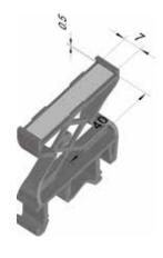
Thanks to the special stop wings, the support can be used both with the adhesive tags provided (together with the product) and with non-adhesive tags of the same size.
