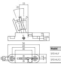
el Material KLF Operation key: stainless steel 304, base: polyamide CPP operation key: stainless steel 304, base: zinc
