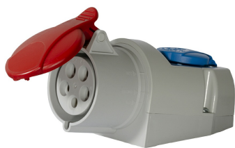
32 A socket contains a 10 A tube fuse to protect the 16 A house socket.
