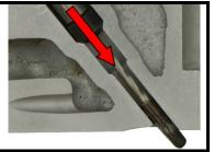
Remove the guide bolt and using suitable tap to make a thread into the glow plug tip.
