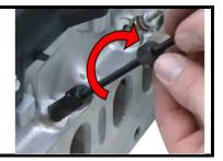
Mount the spindle nut (20 / 21 / 22) onto the extractor spindle and screw the nut against the spindle guide, by using suitable tools.
