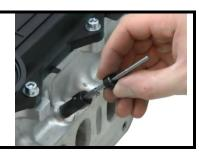
Bore up the glow plug tip with an appropriate twist drill.
