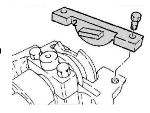
Check that the crankshaft is in 'timed' position and attach Locking Tool to the crankshaft gear using the 3 x M8 Hex.
