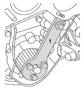
Slacken the belt tensioner and remove the old belt.
