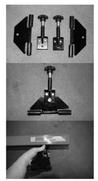
Put a washer on top of the bolt and screw them in place with the help of hand nuts on the engine support.
