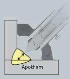
• Determination of the apothem or dimension of the centre for a weld angle.
