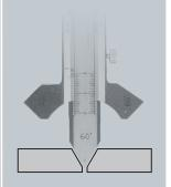
• Evaluation of the angle of a chamfer by comparing the 4 angles on the gauge: 60/70/80/90°
