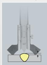
• Determination of the excess thickness of a weld.
