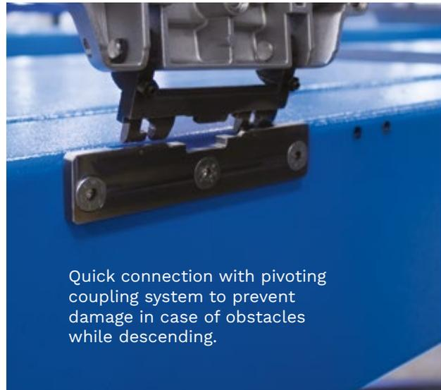
Quick connection with pivoting coupling system to prevent damage in case of obstacles while descending.
