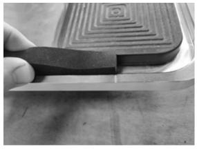
Pinch the gasket into place in the groove. Be careful not to stretch the seal.
