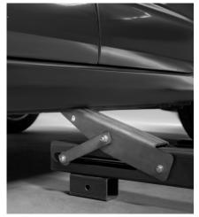
If the area to be straightened is near a wheel, you can use the plate by positioning the vehicle's wheel on the plate. The plate swivels to position itself in the desired pull direction. If necessary, you can add a support using the telescopic extensions.
