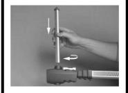
Retract the telescopic measuring arm completely and press the "On/O" on the display panel. A digital number 900 (900mm) will appear in the display window representing the minimum retracted length of the arm between centres.
